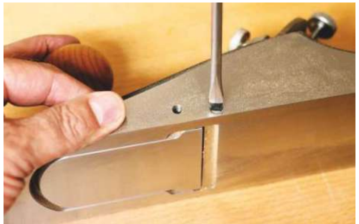
▲ You need a flat screwdriver to nip the side grub screws to the iron
